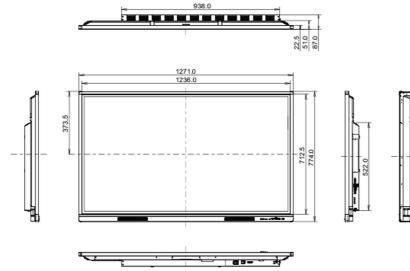
4xM8 SCREW HOLES (VESA MOUNT) Depth=18.5mm-26.0mm [RECOMMEND USING M8-25mm SCREWS]
