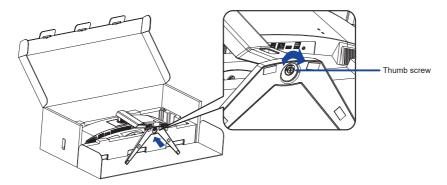
⑤ Carefully take out the assembled monitor from the protecting cushion and stand it up.
