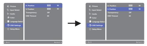
An adjustment page appears after you press the 2 Button. Then, use the 4 7 Buttons to change the vertical position settings. The vertical position should be changing accordingly while you are doing this.
