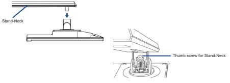
③ Install the Stand-Base to the Stand-Neck and then tighten the 'thumb screw' to secure them.
