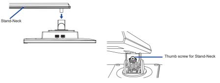
③ Install the Stand-Base to the Stand-Neck and then tighten the 'thumb screw' to secure them.
