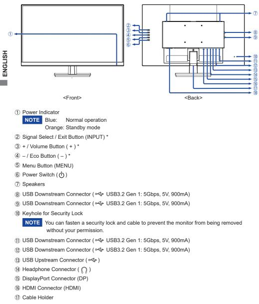
(18) AC Connector (  $\sim$  : Alternating current)
