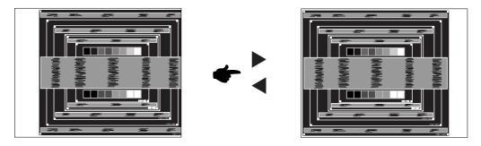
2) Stretch the right side of the picture frame to the right edge of the display area by adjusting the Clock.
