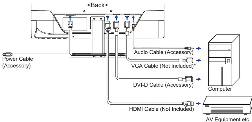
\* VGA cable is not supplied with the monitor. If you use low quality VGA cable, it may cause a result of electro-magnetic interference. Please contact the iiyama Support Centre in your country if you wish to connect the monitor via the VGA input.
