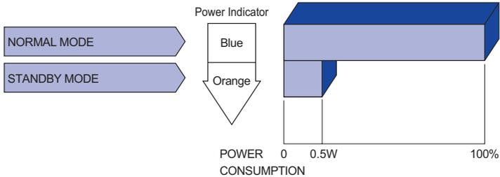
**NOTE** Even when using the standby mode, the monitor consumes electricity. Turn off the Power Switch whenever the monitor is not in use, during the night and weekends, to avoid unnecessary power consumption.
