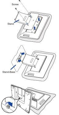
Thumb screw for Stand-Base fixing
