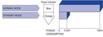
\* When the USB devices are not connected.
