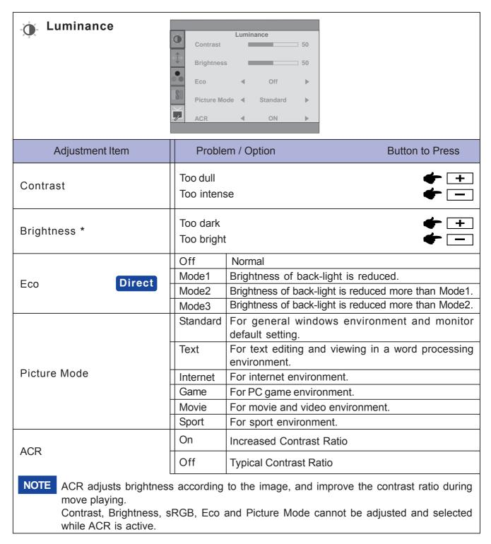
Adjust the Brightness when you are using the monitor in a dark room and feel the screen is too bright.
