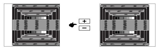
2) Stretch the right side of the picture frame to the right edge of the display area by adjusting the Clock.
