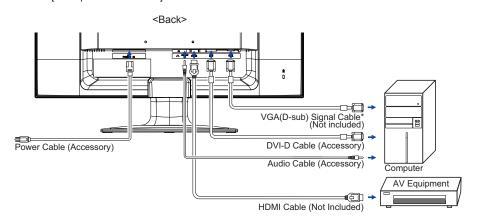
\* VGA (D-Sub) cable is not supplied with the monitor; you need to use a special VGA (D-Sub) cable dedicated for this model. Please contact the iiyama Support Centre in your country if you wish to connect the monitor via the VGA input. Signal Timing
